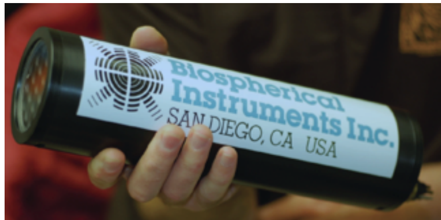
Figure 3 A cluster of 19 micro-radiometers in a pressure housing forms a stand-alone multichannel radiance ocean color sensor that is small enough to hold in one hand.
